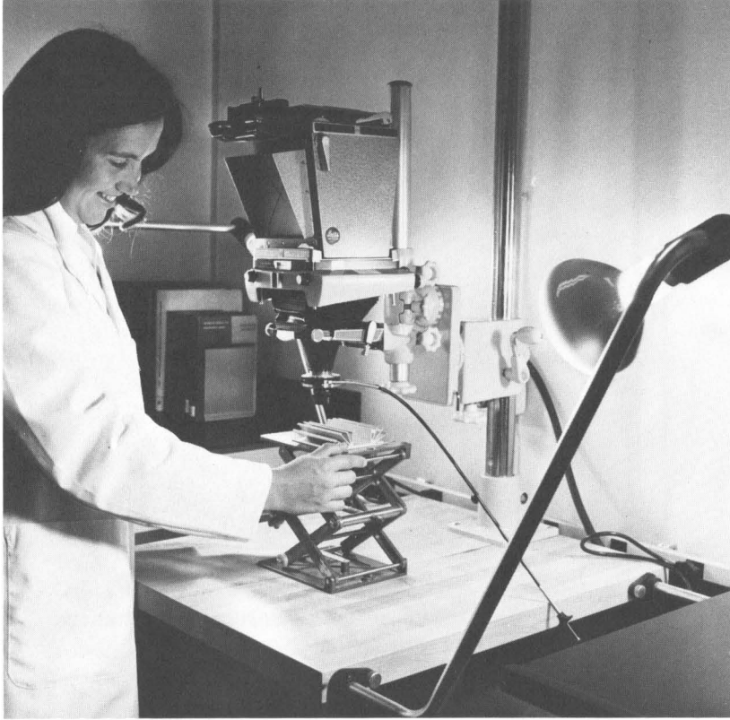
A macrocamera is used to record evidence for failure analysis.
