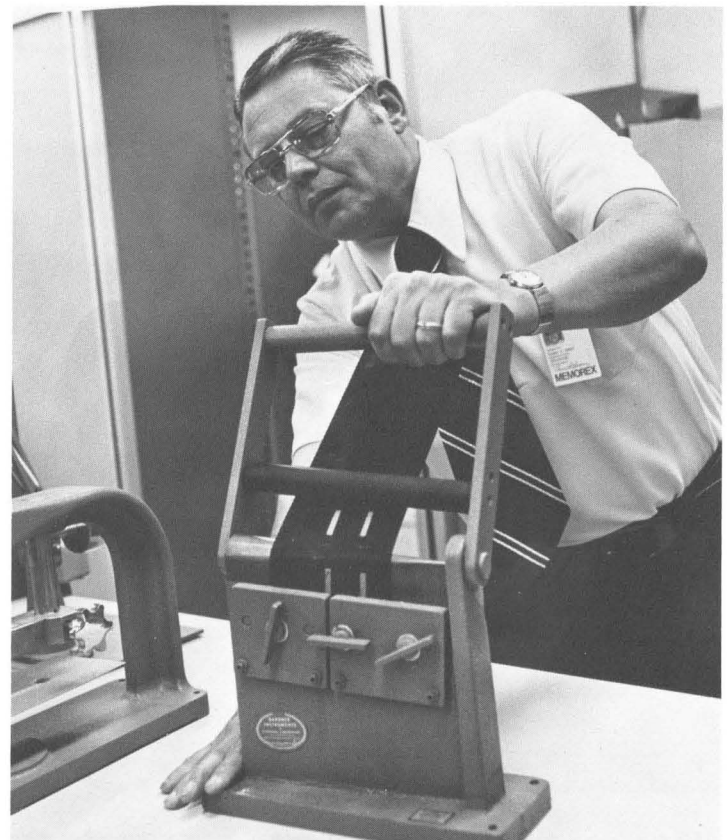
Paint and plating adhesion characteristics can be evaluated.
