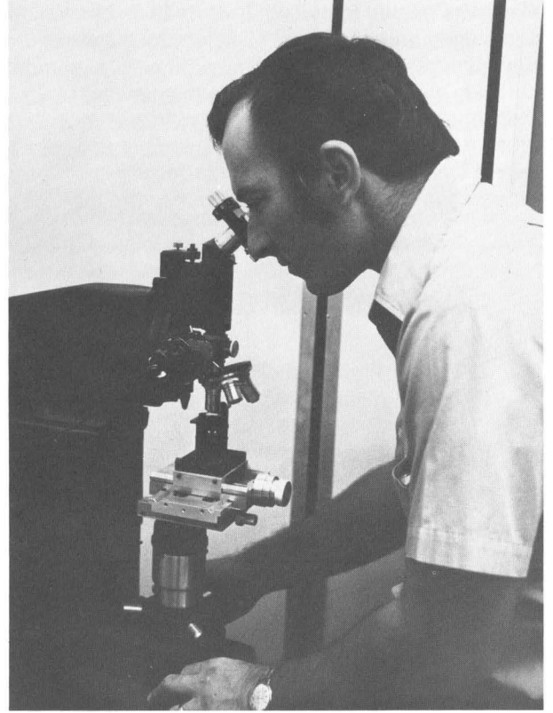
The Tukon microhardness test machine measures the hardness of foil as thin as one mil. It can operate with a load as small as five grams or as heavy as five kilograms.
