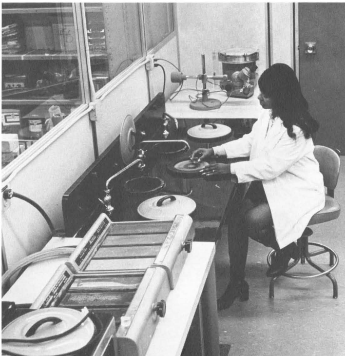
The mount preparation area of the metallurgical section is complete for cross-sectioning, grinding and polishing.
