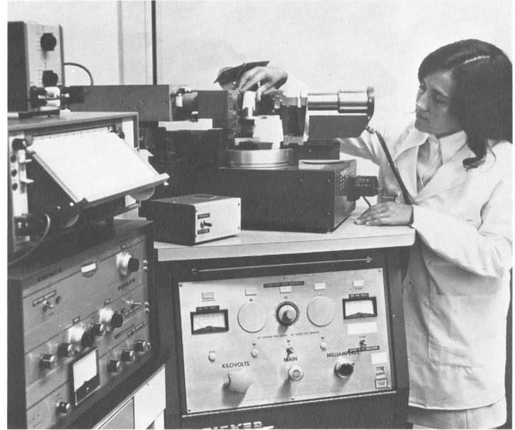
The Picker X-ray Diffractometer can identify compounds, determine residual stress states, measure concentrations and identify many elements.
